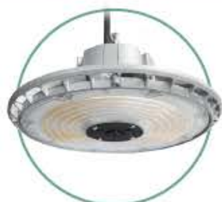
LED High Bay GC350 3CCT Dimerizable 150W/200W 100-277V 4000K - 5000K - 5700K
